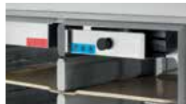
Drawer for enhanced cooling with CO2 pellets during transportation.
